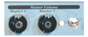
As the name suggests, this controls the overall, global volume of the amplifier. For your enjoyment, there is also a second programmable master volume control, which allows volume adjustments via remote control while you are playing. Both controls are laid out so that even a low-performance effects unit can be used and amplified in the loops.
