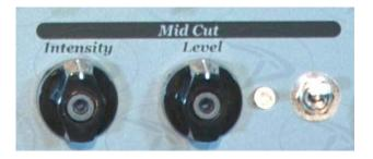
The section Mid Cut incorporates controls for Intensity and Level. Designed for friends of Heavy or Nu-Metal type musical styles, the Intensity control attenuates low midrange at approximately 400Hz. To compensate for the inevitable volume loss when activating this feature, one can bring the volume level back up with the Level Control.
